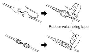
3 Fix both of the coaxial and control cables to protect the inside connections.
