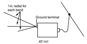
L : Counterpoise length for the operating frequency [m] f : Operating frequency [MHz]
