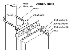
**WARNING:** Mount the AT-141 securely with the supplied nuts and bolts. Otherwise, vibrations and shocks due to waves, etc. could loosen the antenna tuner making if fall, causing personal injury.
